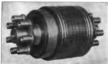
Fig. 4654. Motor Armature and Quill. Westinghouse A. C. Electric Locomotive.
